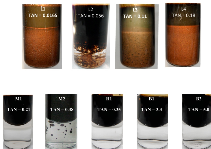
Figure 2. Images of crude oil–water mixtures (1:1 by volume). Images are taken after \sim 24 h of sample preparation. Light, medium, heavy, and extra-heavy crude oils are designated as L, M, H, and B. Total acid number (TAN) is denoted in mg KOH/g oil. All the light oils form water-in-oil emulsions, but in varying quantities (L2 forms the least amount of water-in-oil emulsion, while L1 and L4 form the most amount of water-in-oil emulsion). No emulsion formation is observed in the medium, heavy, and extra-heavy oils.
