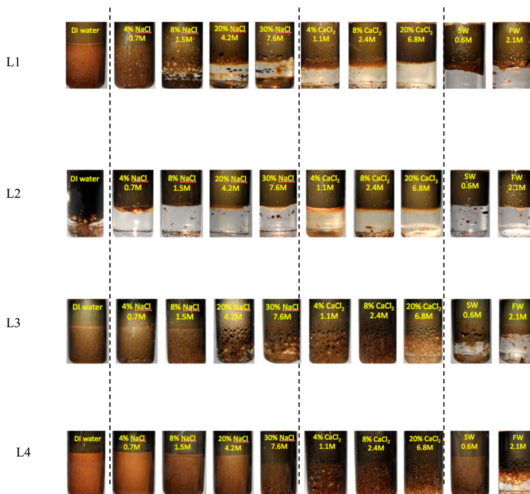
Figure 4. Images of crude oil–brine mixtures (1:1 by volume) for all the light oils. Images are taken after ~24 h of sample preparation. Brine is characterized by various concentrations of NaCl, CaCl 2 , and two multicomponent salt solutions SW and FW (concentrations indicated in wt % and ionic strength in mol/L).
