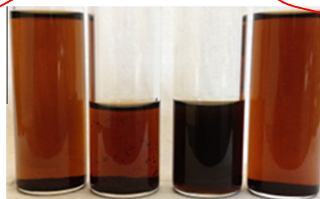
Fig. 7. Addition of TEA. From left to right, the mixtures are at c = 0 with TEA, c = 0 without TEA, c = 1000 ppm DBSA without TEA, and c = 1000 ppm DBSA with TEA. All four mixtures are composed of QAB.
